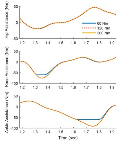
Figure 2. Torque profiles vs magnitude of assistance
