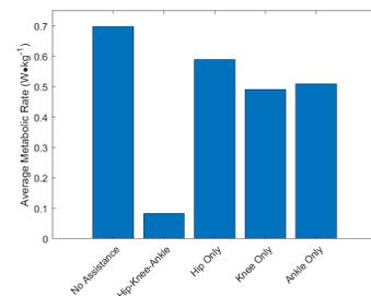
Figure 6. Metabolic cost reductions single-joint vs multi-joint
