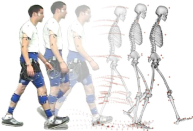
Experimental markers are matched by model markers throughout the motion by varying the generalized coordinates (e.g., joint angles) through time. See [Inverse Kinematics](#) for full documentation on running IK in OpenSim. [Tutorial 3 - Scaling, Inverse Kinematics, and Inverse Dynamics](#) walks through an example of using Inverse Kinematics for human walking.
